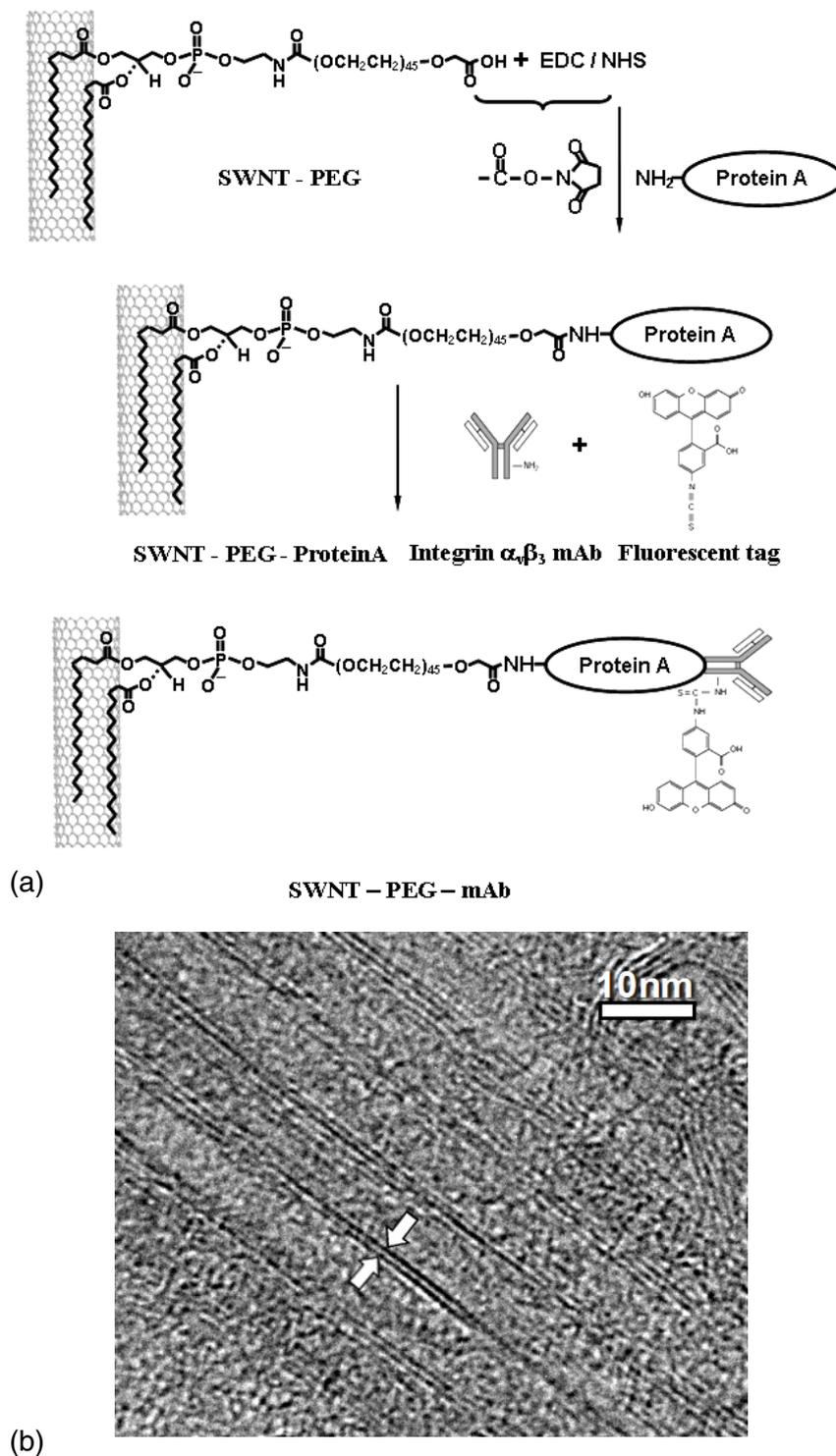
**Figure 1.** (a) An illustration of the procedures of producing SWNT-PEG-mAb. (b) A typical TEM image of SWNT-PEG.
