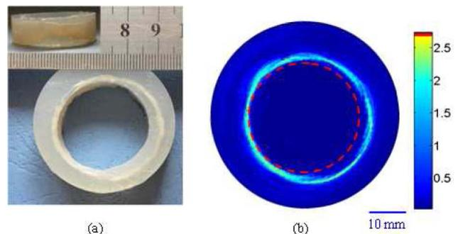
Fig. 2. (Color online) (a) Photograph of the *ex vivo* pig colorectal tissue embedded in the transparent gelatin phantom. (b) Reconstructed PA tomography of pig colorectal wall.
