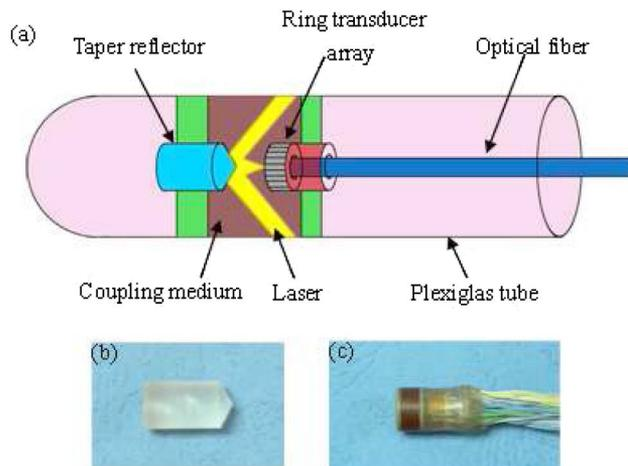
Fig. 1. (Color online) (a) Schematic of the PAIE. (b) Photograph of the taper reflector. (c) Photograph of the hollow ring transducer array.
