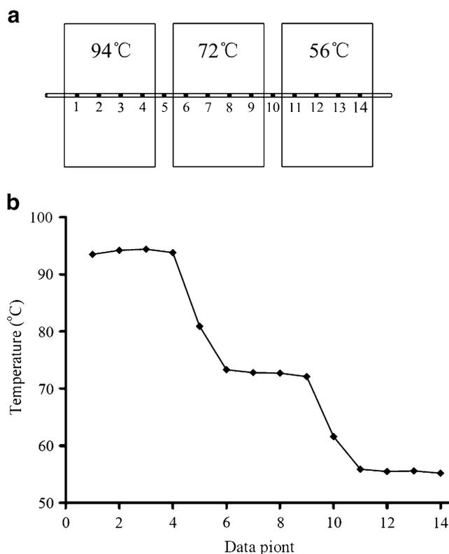
**Fig. 2** a Schematic drawing of temperature data points along the microchannel. b Temperature distribution in the microchannel. Data at each point was measured five times
