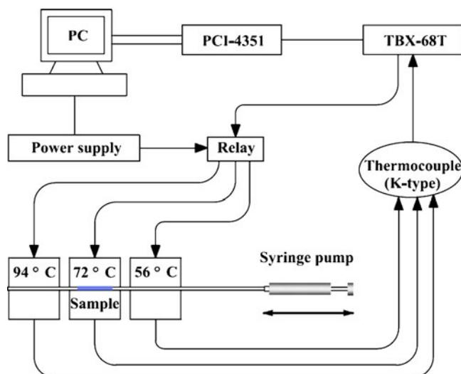
**Fig. 1** Schematic diagram of the oscillatory-flow multiplex PCR microfluidics
