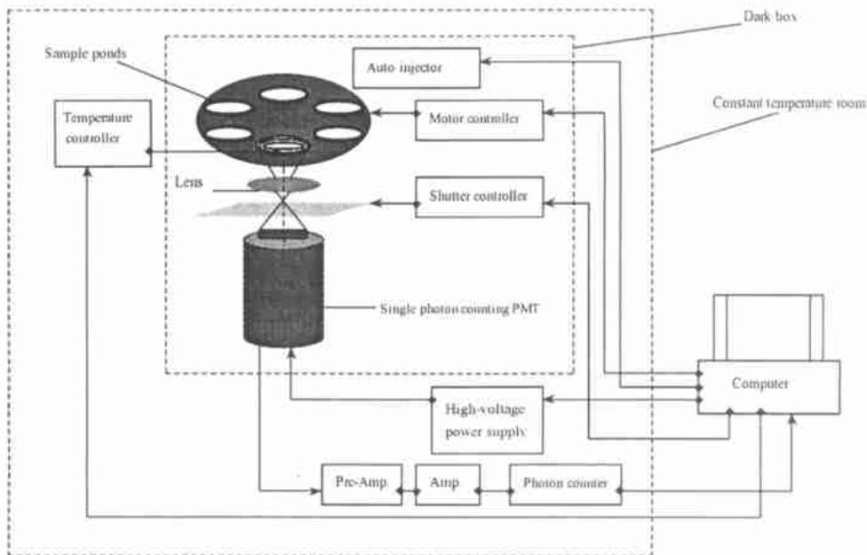
**Fig. 1** A schematic representation of the single photon counting system for measurements of CL. Constant temperature room was 25 °C, relative humidity was 65%.
