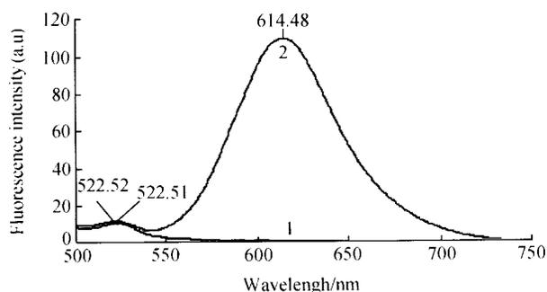
Fig. 1. The fluorescence emission spectrum of  $\text{Ru}(\text{bpy})_3^{2+}$ . 1, the fluorescence emission spectrum of DMF using an excitation wavelength of 456 nm; 2, the fluorescence emission spectrum of  $\text{Ru}(\text{bpy})_3^{2+}$  dissolved in DMF using an excitation wavelength of 456 nm.
