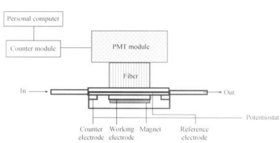
Fig. 2. A diagram of the essential components of the instrument.
