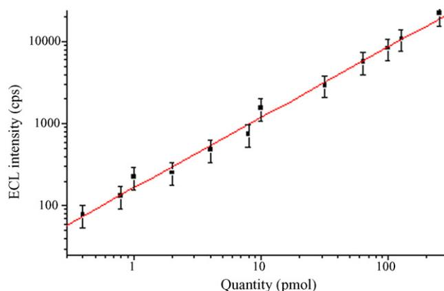
Fig. 2. Calibration curve for the ECL system: the calibration curve was obtained by measuring different quantity of labeled DNA. The minimum detectable quantity was 100 fmol. The curve shows a profile with a linear region from 0.1 to 250 pmol ( $R^2 = 0.997$ ). This wide dynamic range is useful in developing quantification assay.
