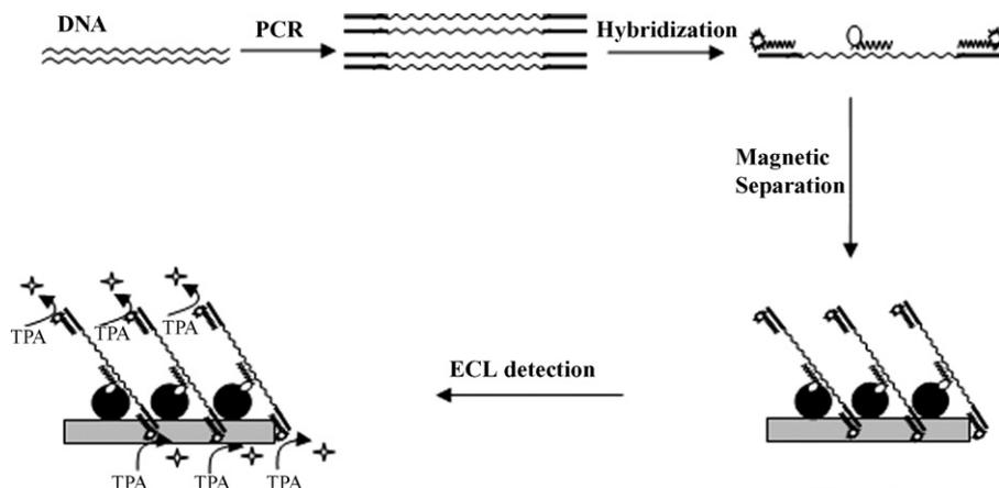
Fig. 1. The basic principle of the improved ECL-PCR method for detection of plant viruses: TBR-probe (★); biotin-probe (●); magnetic beads (●); photon (★).
